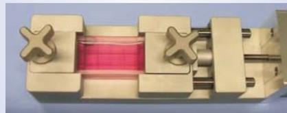
Mechanical stimulation device to strain a silicone dish with adherent growing cells.
