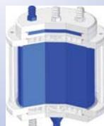
Fig.5: Aerated extracapillary space (ECS) for biofilm formation and product recovery.
