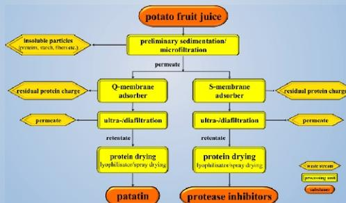
Figure 3: Flow-chart of PFJ processing
