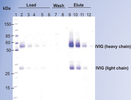
Fig.3 Purification of IVIG via Sartobind Protein A Direct from cell culture suspension (12% SDS-Gel).
