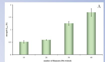
**Figure 3:** Mechanical properties of spider silk strand. A: maximal strength B: elongation at break
