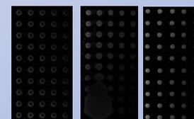
Figure 2: First five dilutions on a FAST slide with Next Spot PB, from left to right: pin and ring, split pin, non-contact printer.
