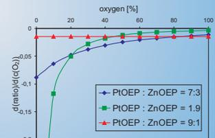
Fig. 5: Oxygen sensitivity of different mixtures of PtOEP and ZnOEP
