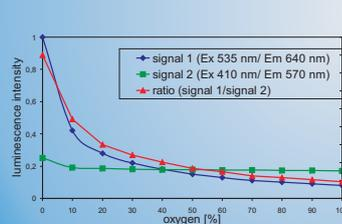
Fig. 4: Oxygen dependence of luminescence signals and Ratio, PtOEP:ZnOEP = 9:1
