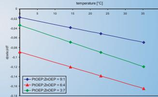
Fig. 7: Temperature sensitivity of different mixtures of PtOEP and ZnOEP
