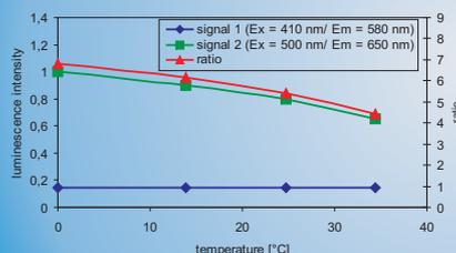
Fig. 6: Temperature dependence of luminescence signals and ratio, PtOEP:ZnOEP = 1:9
