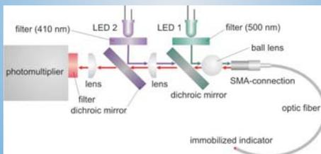
Fig.3: Optical set-up of the sensor
