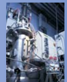
reactor cultivation (10 L scale)
