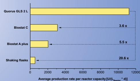
Fig. 3: Average production rate of a recombinant protein per reactor capacity in various cultivation vessels while cultivation of *A.niger*.
