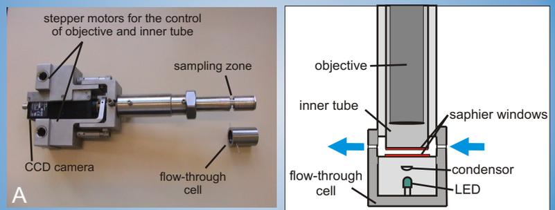
Figure 1: Photo (A) and schematical drawing (B) of the In-situ microscope and the flow-through cell covering the sampling zone.
