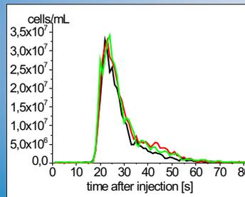
Figure 3: FIA result peaks for a deployed cell density of  $1.5 \cdot 10^8$  cells/mL
