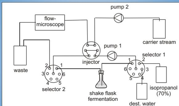
Figure 2: Automated FIA system used to inject a sample (500  $\mu$ L) from a shake flask fermentation into a carrier stream, which is transported to the flow-microscope for image analysis. It also enables automated sterilization and cleaning.
