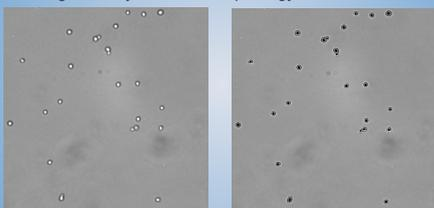
Figure 5: Image and resulting image of yeast cells (390x magnification). The image analysis system detected 24 kernels making 18 single cells and 3 double cells. The cell density is determined from the number of kernels divided by the sampling zone volume ( $0.0101 \text{ mm}^3$ ) resulting in  $2.4 \cdot 10^8$  cells/mL.
