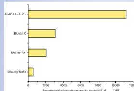
Fig. 5: Average production rate of a recombinant protein per reactor capacity in various cultivation vessels while cultivation of *A.niger*.
