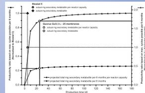
Fig. 8: Modelling of a Quorus GLS cultivation of *S.coelicolor* to produce a secondary metabolite. Effect of increasing Quorus GLS production time up to 180 days onto the total product output and space-time-yield to estimate the break-even with a Biostat C. All values are normalized to the accumulative output of the maximum number of Biostat C batches in 180 days.
