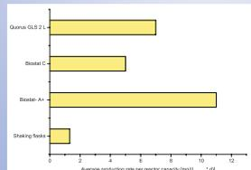
Fig. 7: Average production rate of a secondary metabolite per reactor capacity in various cultivation vessels while cultivation of *S.coelicolor*.
