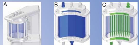
Fig. 2 A: Quorus GLS disposable bioreactor unit. B: Aerated extracapillary space (ECS) for biomass formation and product recovery. C: Intracapillary space (ICS) for nutrient supply.
