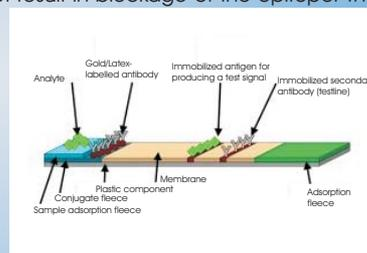
Fig. 3: Schematic setup of a dipstick immuno assay
