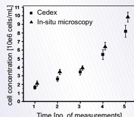
Figure 5: Cell density during the cell accumulation phase as determined by Cedex and In-situ microscope
