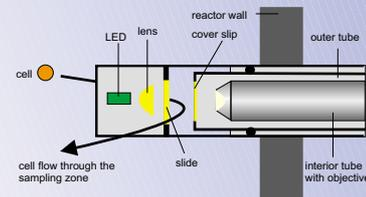
Figure 2: The sampling zone of the in-situ microscope
