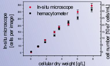
Figure 5: Linear dependency of hemacytometer offline and in-situ microscope online counting
