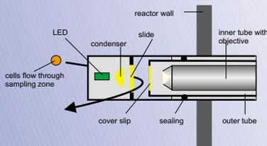
Figure 3: Flow-through sampling zone of the in-situ microscope
