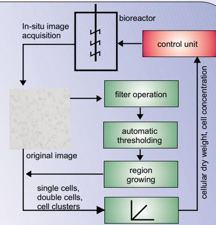
Figure 4: Integration of yeast cell image analysis into the process control
