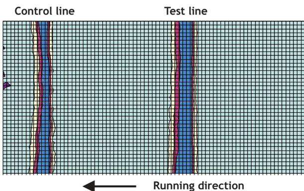
Figure 2: Miscoloured plot of an analysed dipstick test. The darker the colour the more intensive are the lines. It is obvious that the test line is much thicker than the control line. Both lines are inhomogeneous coloured.
